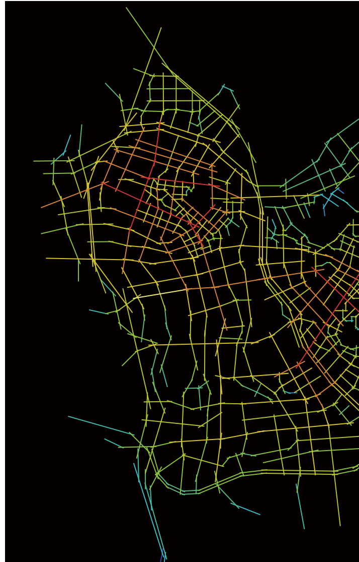
Figure 12. The space syntax map of the road network in the Guangming New District master plan (2007-2020). Local Integration [R3]; The integration of the Guangming New District when the direction is changed 3 times.
