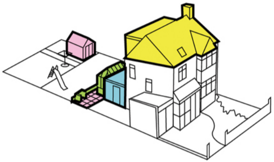
1990 the loft extension gives that extra room...and an ensuite
